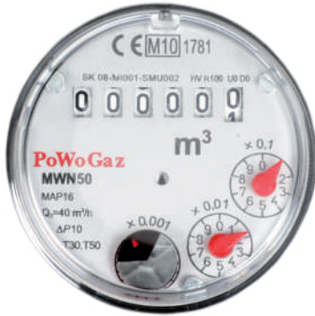
IP 65 dial and barrel counter, complete with a retro-reflective pointer and contained in a plastic housing. Preequipped for interfacing with data transmission modules.
